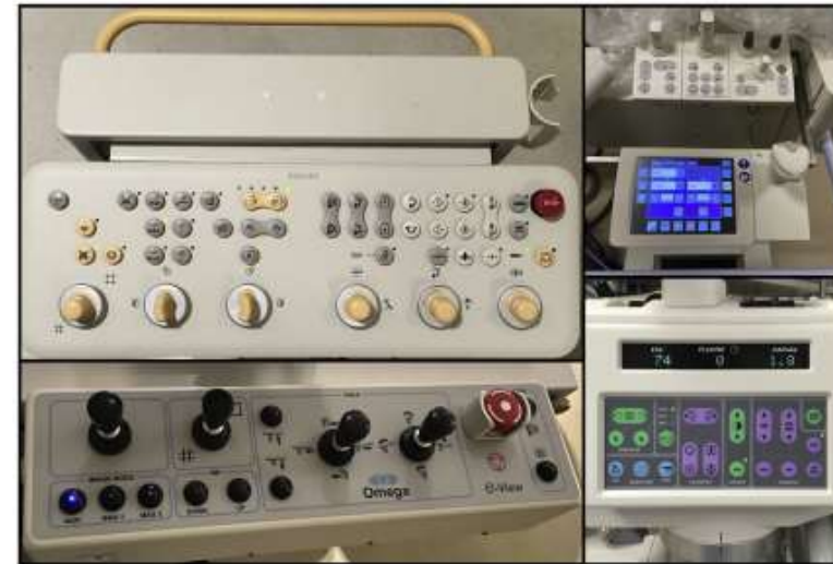
Figure 1. Representative control panels from 4 different fluoroscopy manufacturers. Note the lack of standardization of key controls. Clockwise from upper left: Philips (Amsterdam, Netherlands), Siemens Healthineers (Erlangen, Germany), GE Healthcare (Chicago, Illinois), Omega Medical Imaging (Sanford, Fla, USA).
